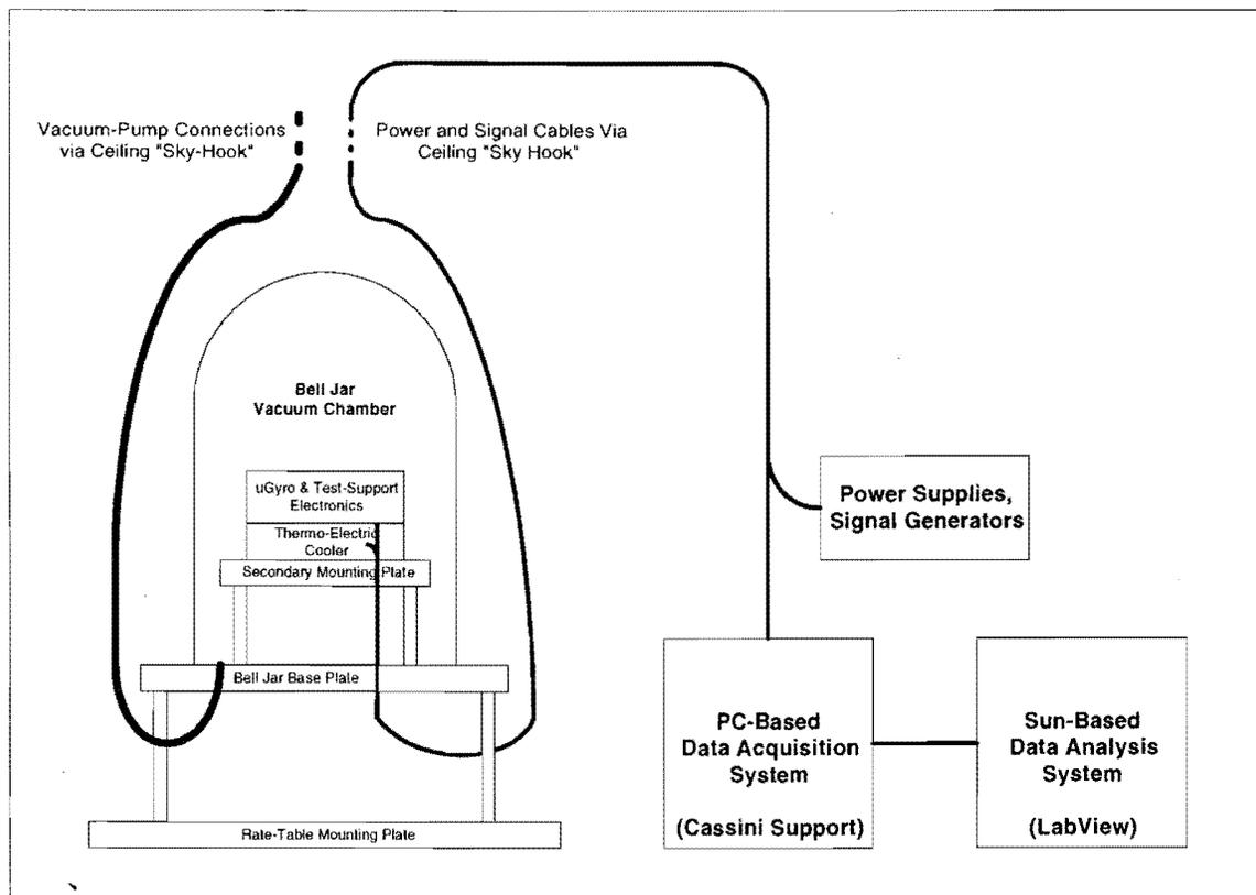
Figure 1. Microgyro Test Configuration.
