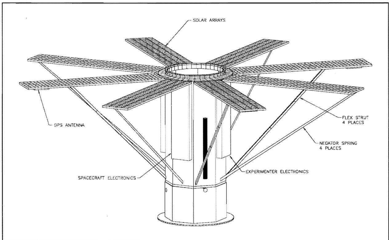
Figure 5 - Solar Pointing SPARTAN LITE (Side 1)
