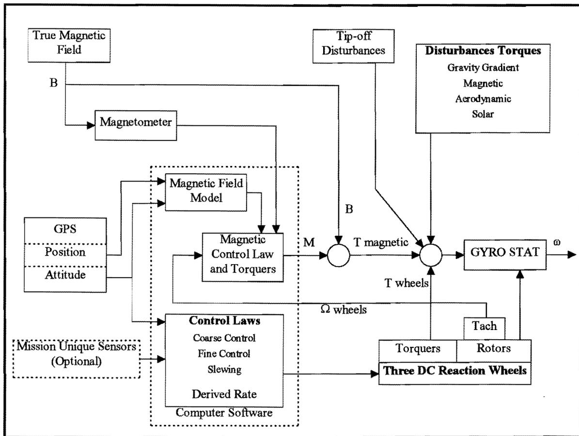
Figure 10 ACS Block Diagram
