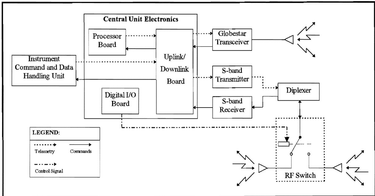
Figure 11 RF Communication Subsystem
