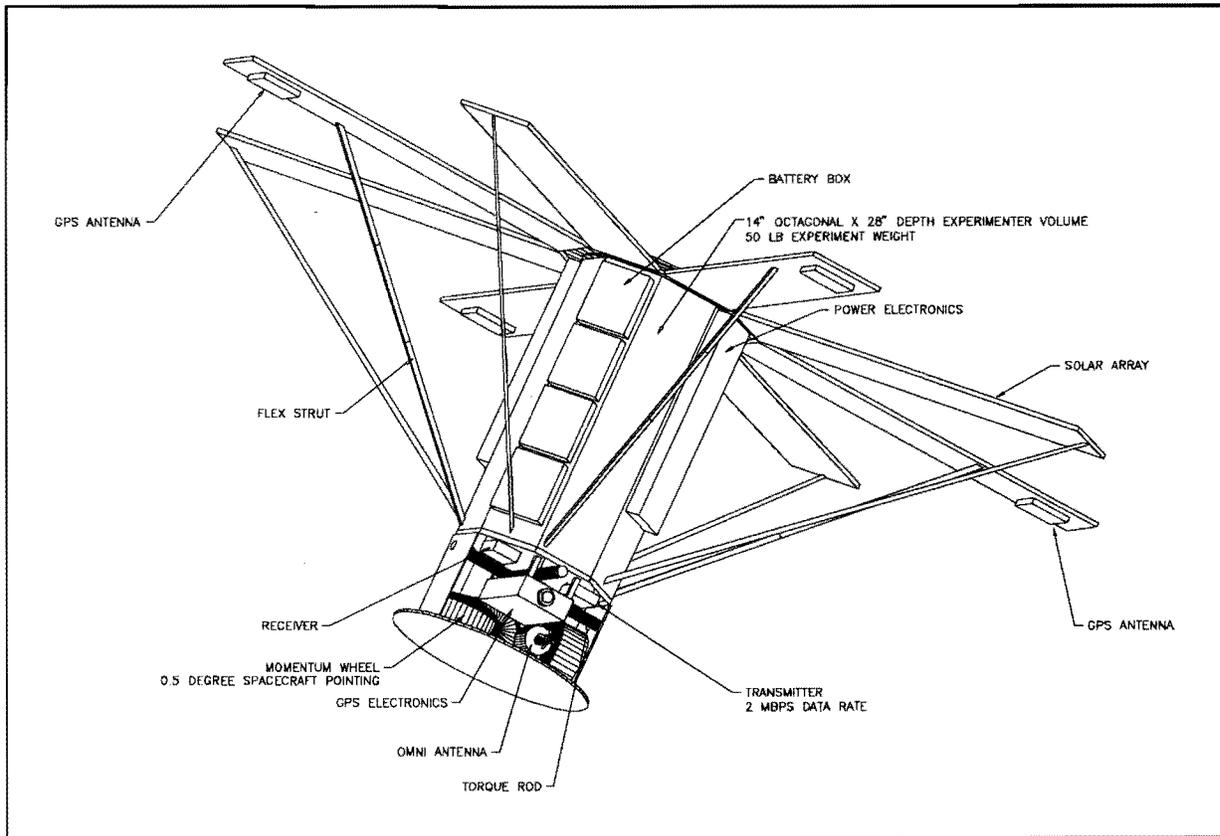
Figure 6 - Solar Pointing SPARTAN LITE (Side 2)
