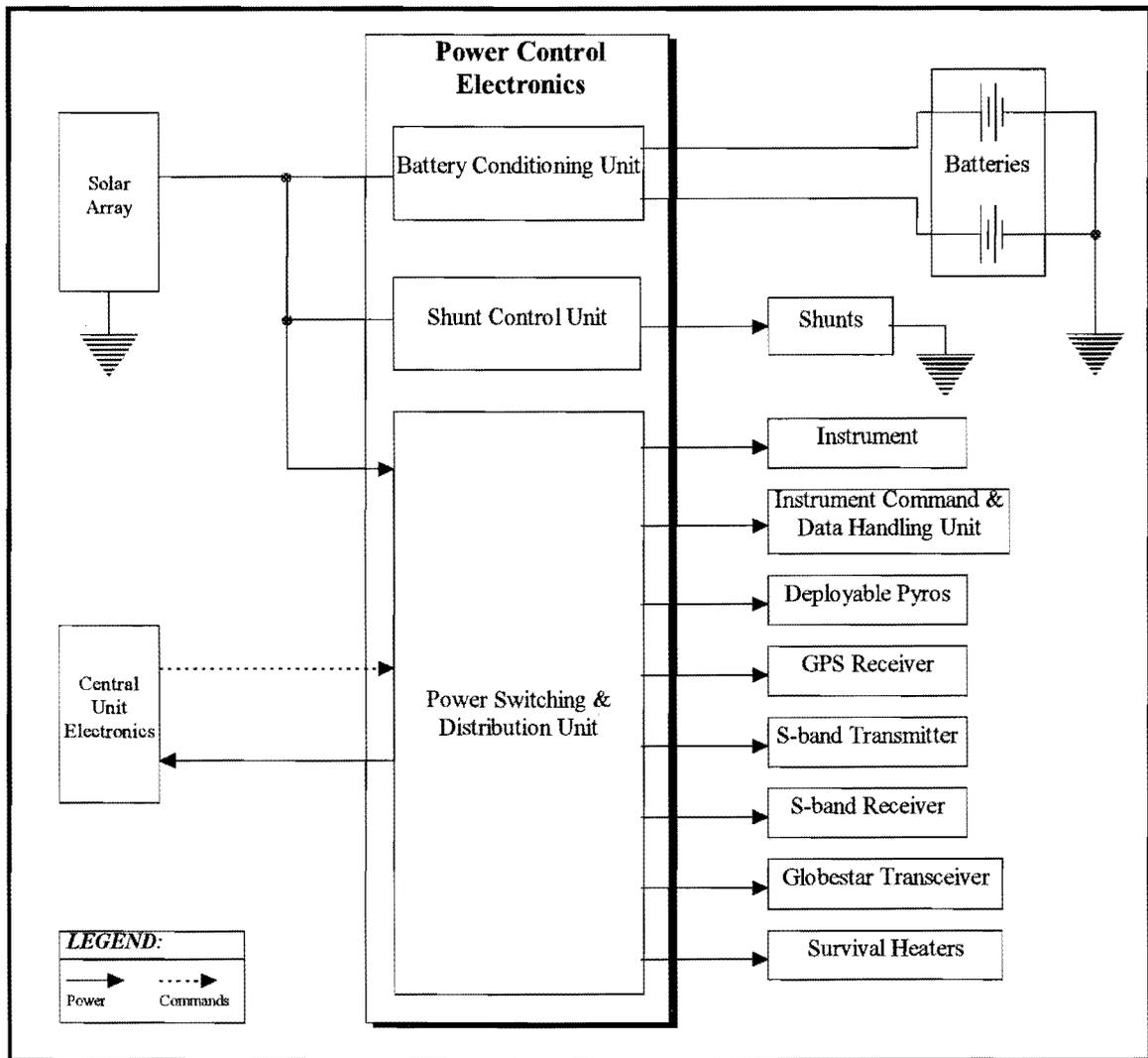
Figure 9 Power Subsystem Block Diagram
