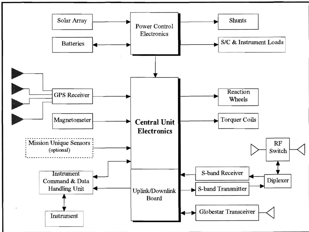
Figure 7 SPARTAN LITE Block Diagram
