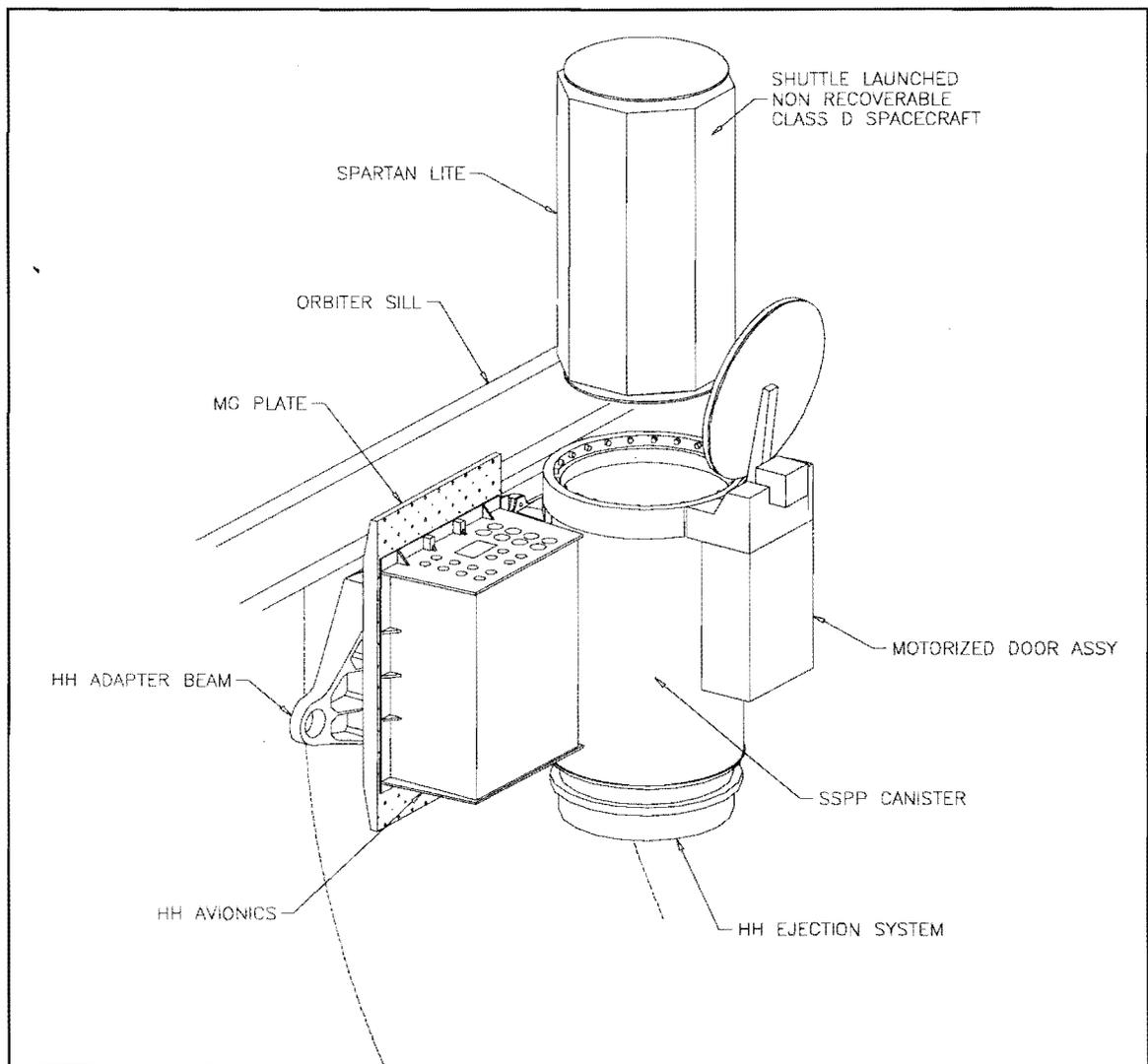
Figure 1 - SPARTAN LITE Sidewall Configuration
