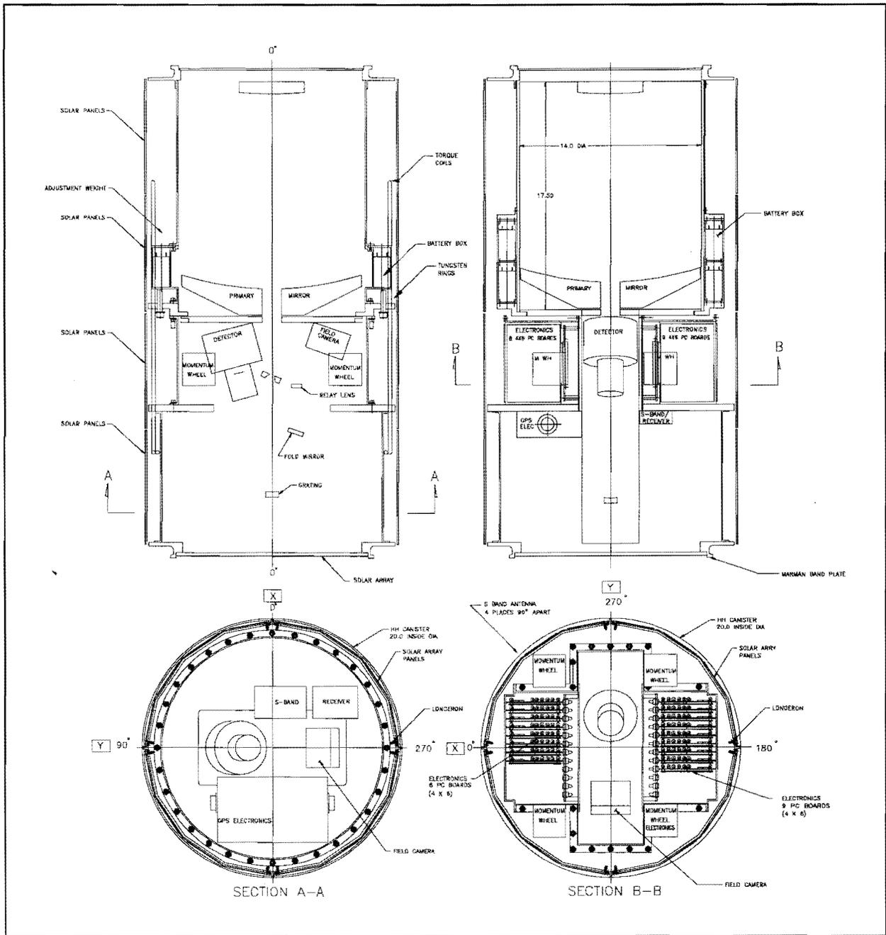
Figure 3 - ASTRO HITCHHIKER Component Placement
