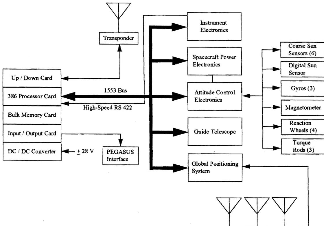
**Fig. 2. TRACE Data Flow Diagram**
