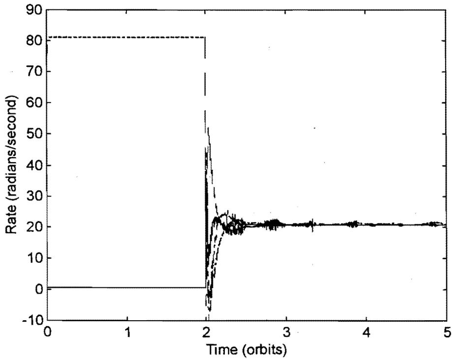
Fig. 11. Reaction Wheel Speeds
