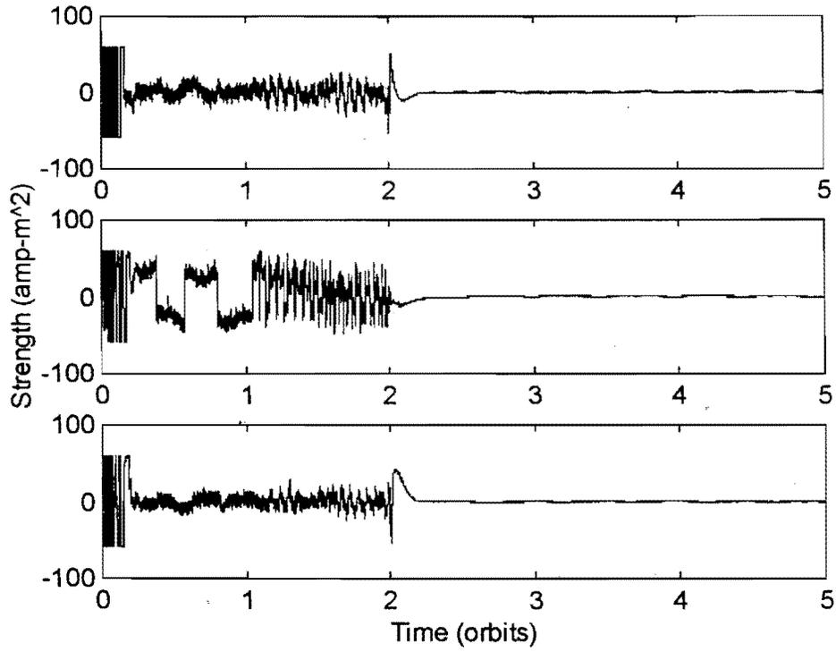
Fig. 10. X, Y and Z Torque Rod Dipole Commands
