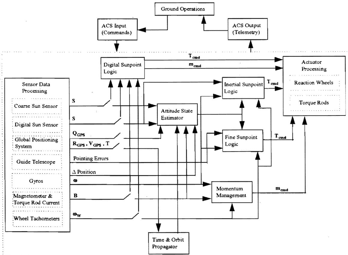
Fig. 7. TRACE Software Architecture
