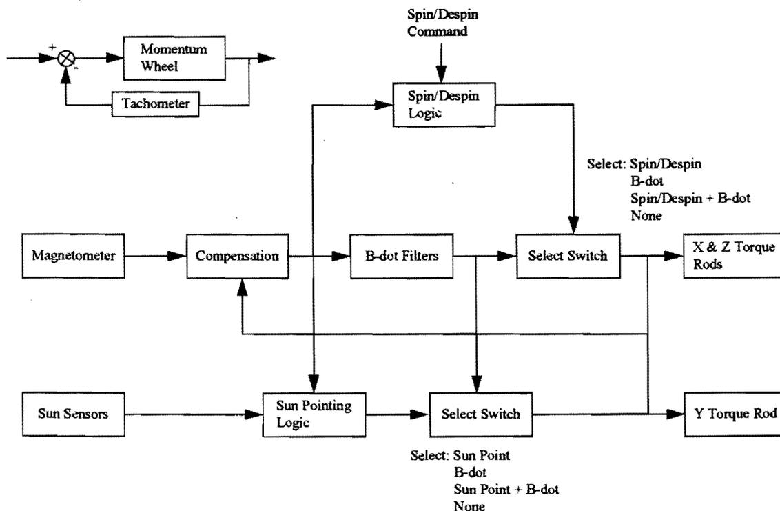
Fig. 3. Acquisition/Safehold Mode Block Diagram
