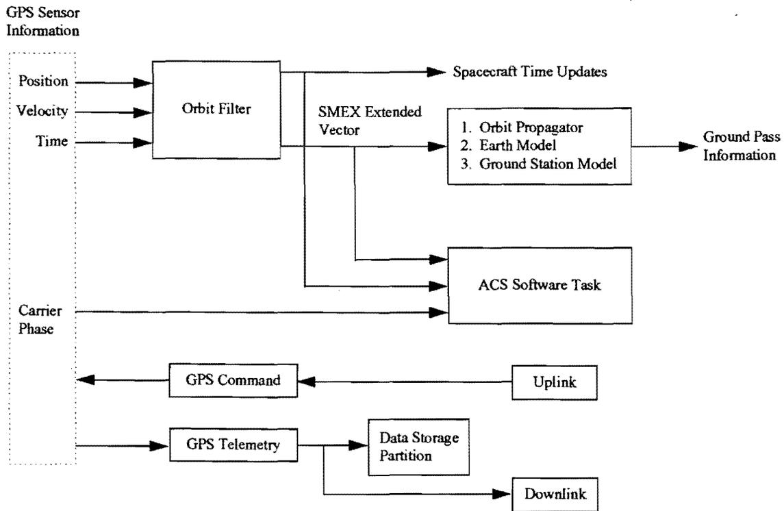
**Fig. 6. GPS Task Architecture**
