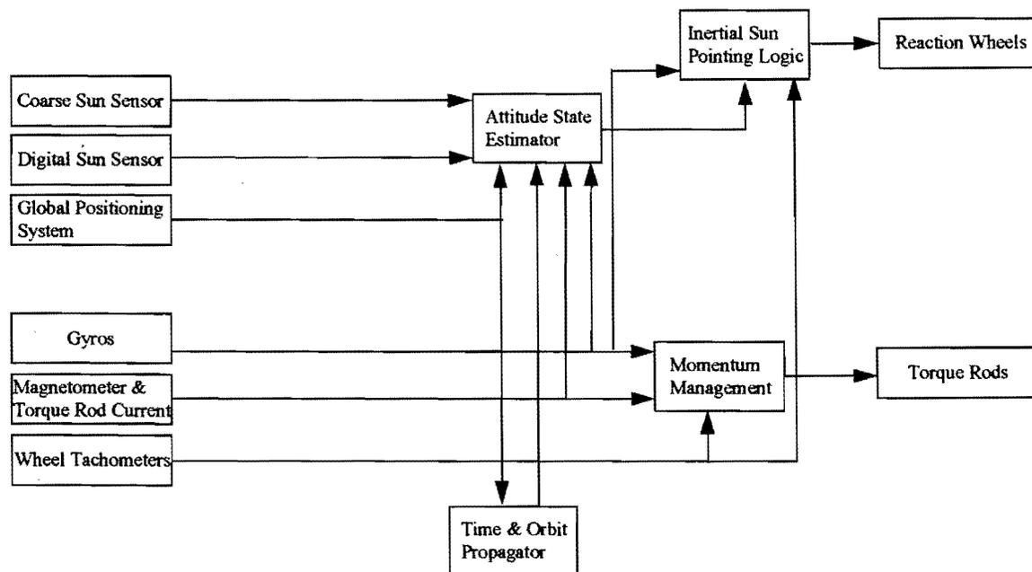
Fig. 4. Inertial Sunpoint Block Diagram
