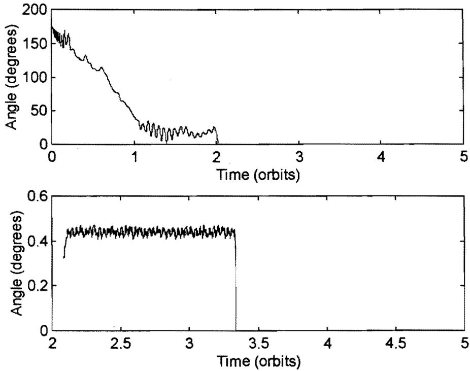
**Fig. 8. Angle Between the Instrument Boresight and the Sun Line**
