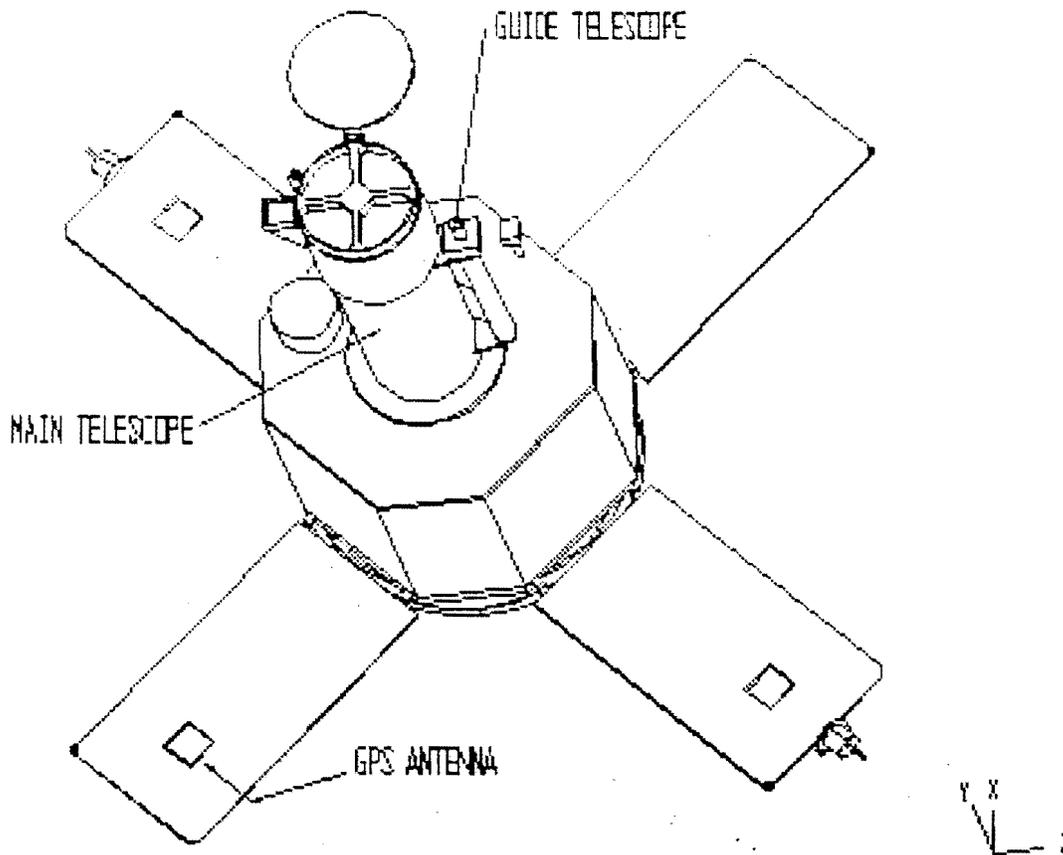
Fig. 1. Fully Deployed, On-Orbit TRACE Satellite Configuration
