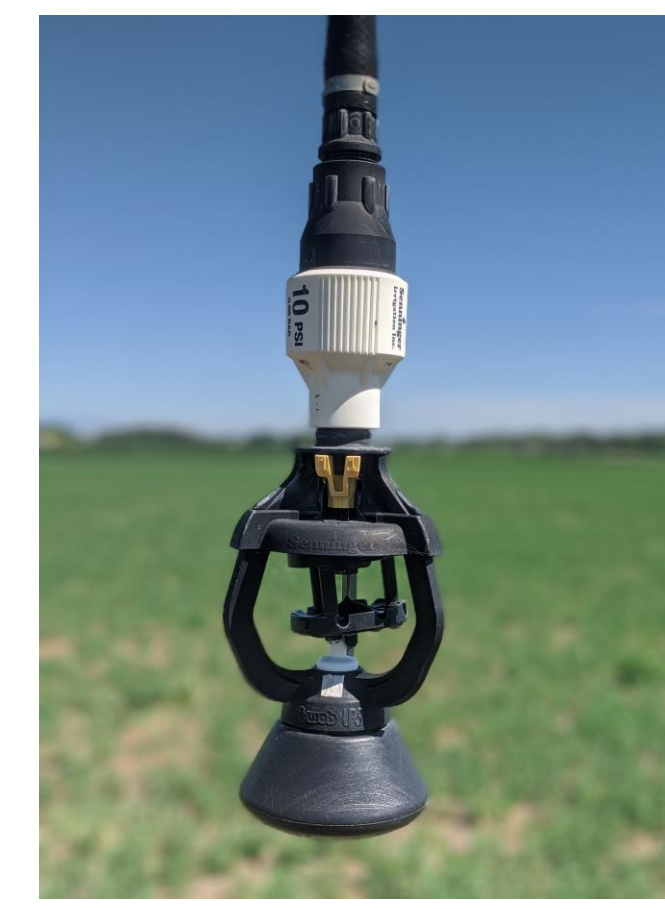
MESA Nozzle 78% irrigation efficiency 20-75 ft wetting diameter 3-6 ft above soil surface 7.5-20 ft spacing between drops
