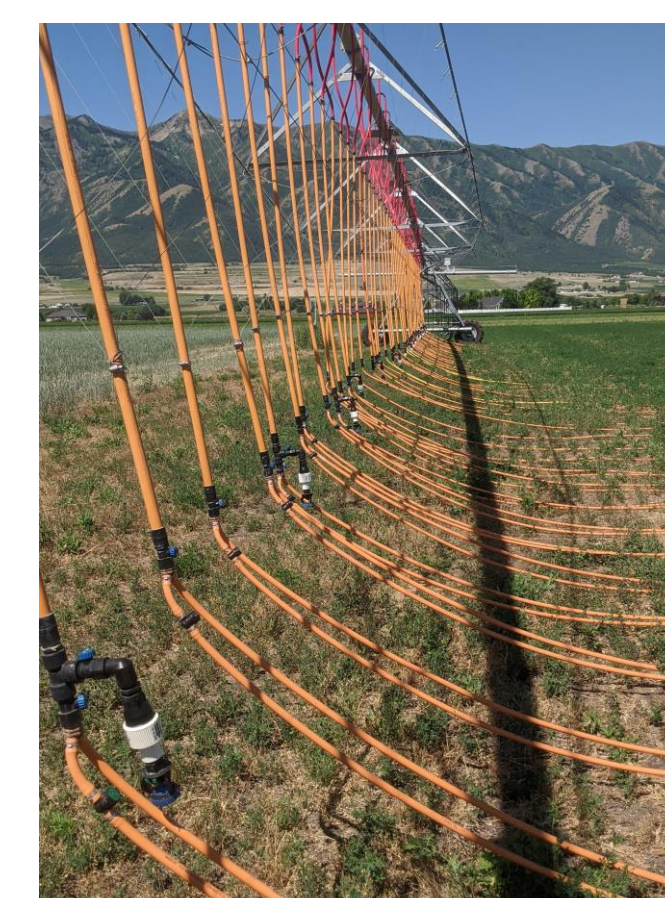
MDI Lines 97% irrigation efficiency 1-2 gallons per hour every 6 inches 1.5-3.5 ft between lines
