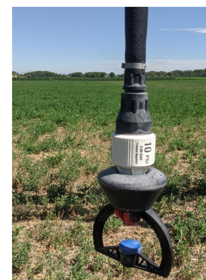
LEPA Nozzle 88% irrigation efficiency 12-30 ft wetting diameter 1-3.5 ft above soil surface 2.5-5 ft spacing between drops
