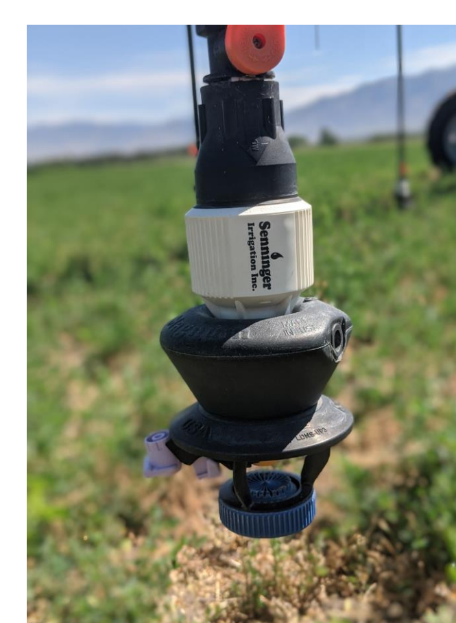
LEPA Nozzle 95% efficient, various parts to change angling of water 1-2ft above soil surface 2.5-3.5ft between drops
