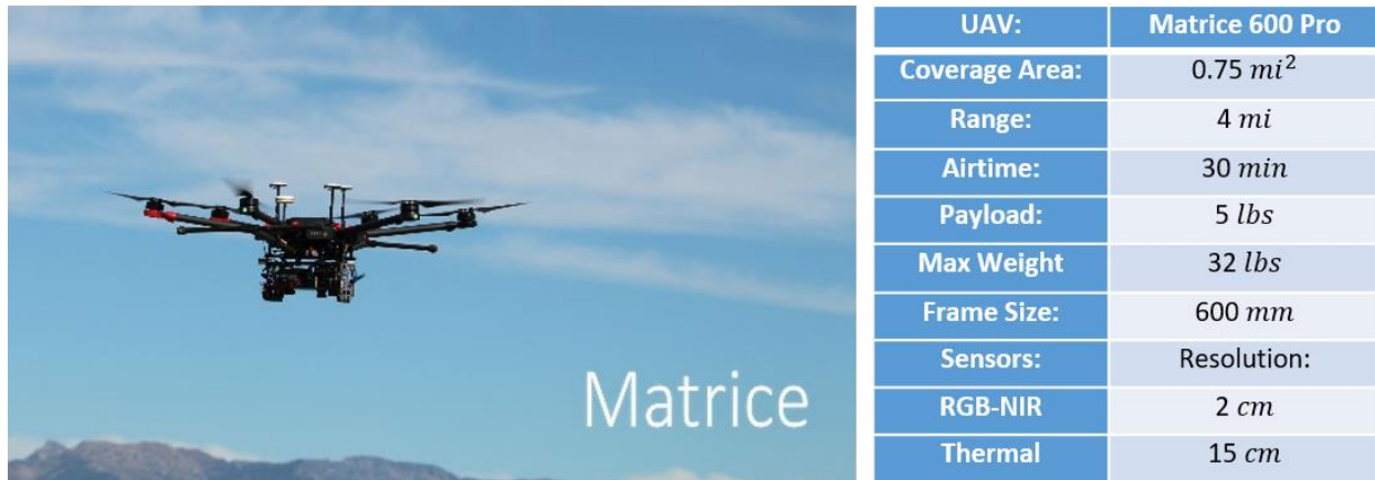
Figure 3: Specifications of the Matrice 600 Pro octocopter, which conducted the UAV flight ( https://uwrl.usu.edu/aggieair/uav-service-center/platforms-sensors ).
