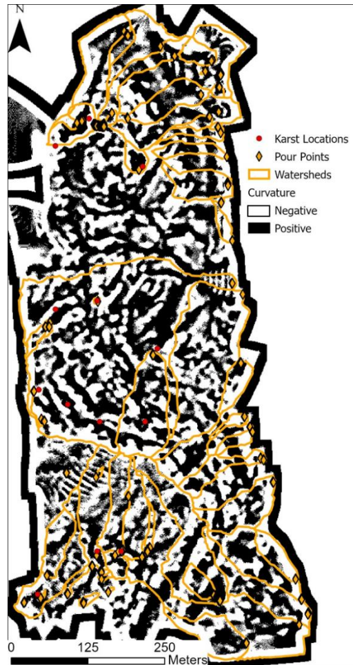
Figure 23: Calculated pour points and delineated watersheds on top of a curvature layer. Watersheds and pour points were calculated using focal statistics with a 3 \times 3 rectangular matrix used to calculate mean values. The curvature layer was calculated using T = 5 and dt = 1 .
