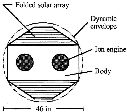
Figure 2. Rear view of the spacecraft in the launch vehicle dynamic envelope
