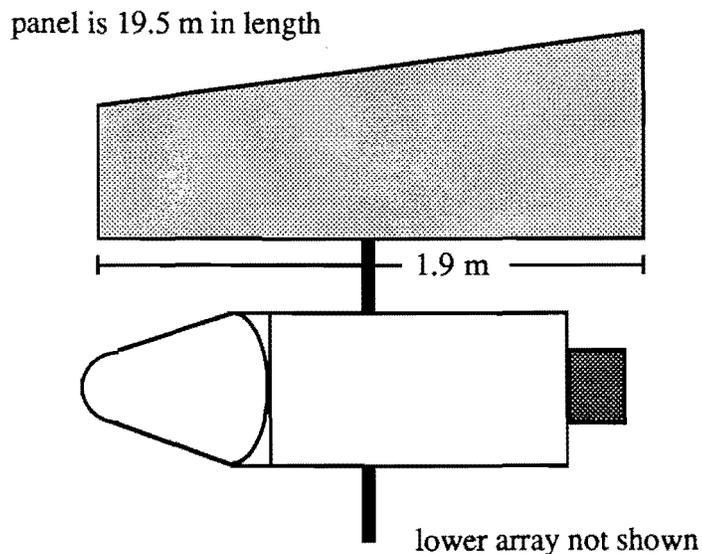
Figure 3. Side view of the spacecraft in orbit after array deployment
