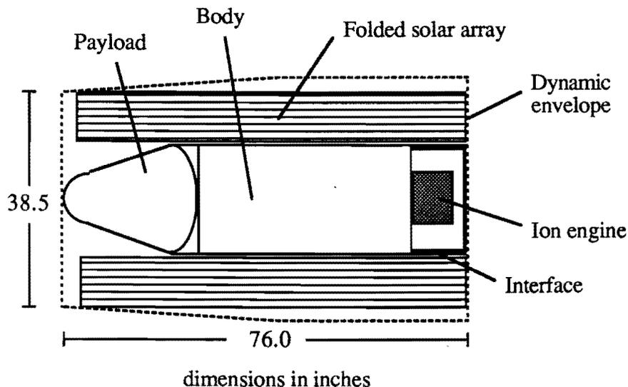
Figure 1. Side view of the spacecraft in the launch vehicle dynamic envelope
