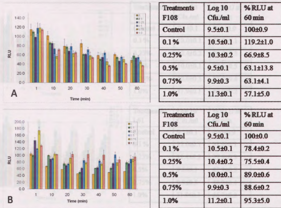
Figure 25: Lux response (A) slight effect (B) activation of P. putida KT2440 biosensor to F108 Pluronic at defined doses (mg/L). Changes in Lux output relative to control and cell culturability after 60 min of treatment are shown. Means of analytical results and standard errors are shown.
