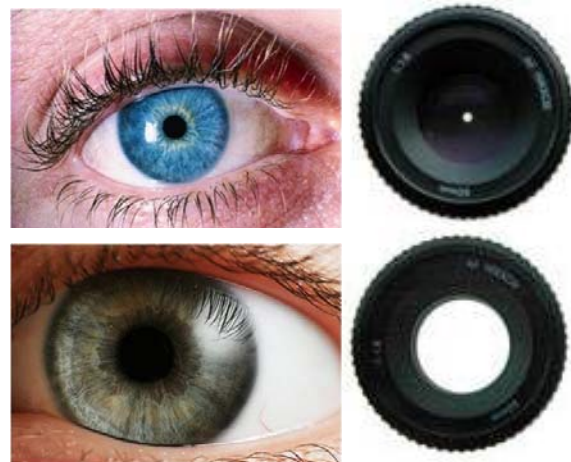
Figure 1. This diagram compares a diaphragm aperture's function in relation to the pupil of an eye.
