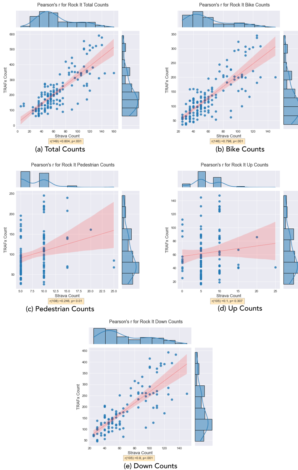
Figure C.6: Pearson's r correlation plots summarizing relationship between Strava Metro and TRAFx total, bike, pedestrian, up, and down counts for the Rock It trail.
