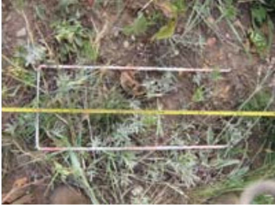
Figure 7. Daubenmire quadrats measure herbaceous cover.
