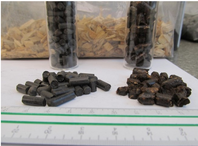
Figure 4. Biochar pellets (left) produced using high-temperature pyrolysis compared to pellets made from torrefied wood (right) Photo Credit: Nate Anderson, USDA Forest Service
