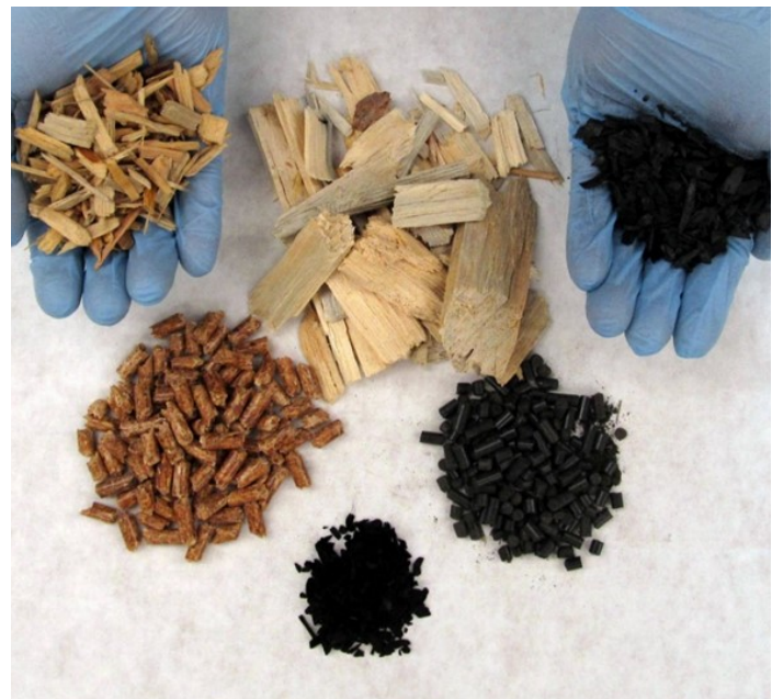
Figure 3. Five pyrolysis products plus pulp chips. Clockwise from top left: microchips from mixed conifer woody biomass, 3-inch pulp chips for reference (center), high carbon biochar resulting from pyrolysis at 1,000°C, pellets made from char, high surface area activated carbon made from char (biochar), and pellets made from wood. Photo credit: Nate Anderson, USDA Forest Service
