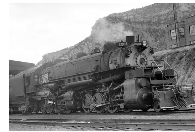
Figure 8: Utah RY Locomotive, engine number 201, engine type 2-8-8-0 Photograph by Otto Perry in 1935.
