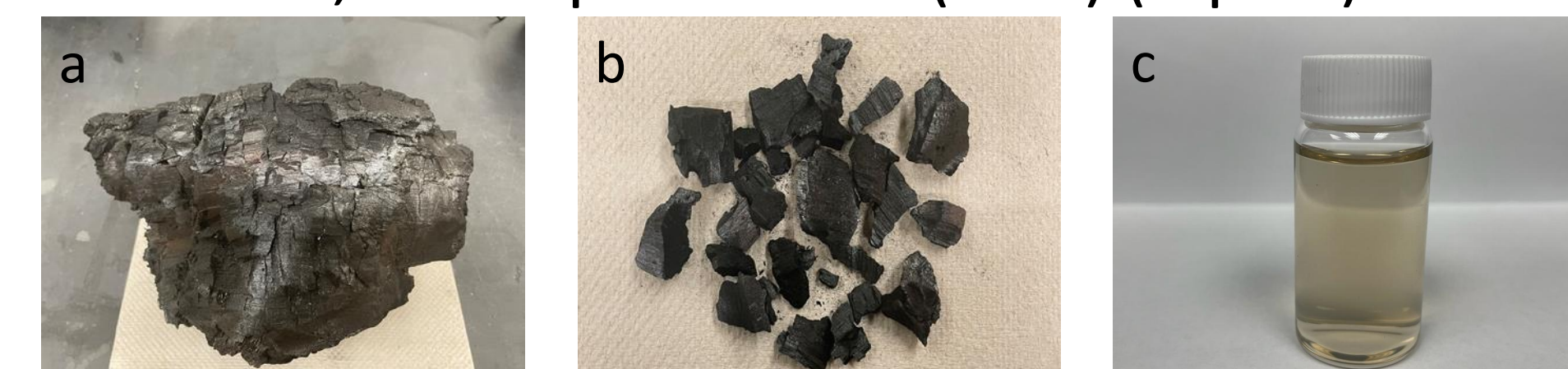
Figure 2. (a) Collected sample portion. (b) Chipped off pieces from the sample. (c) Obtained pyDOM solution after grinding, sieving, agitation, centrifugation and filtration.
