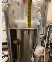
Figure 2: Height of the foam reduced after the inverted cone was connected to the inner shaft
