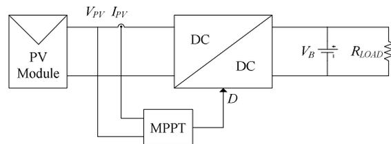
Figure 1: Block diagram of a MPPT technique
