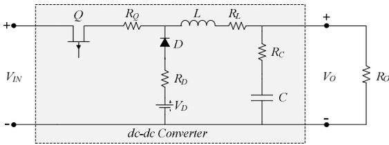
**Figure 2: Buck converter model including device losses**
