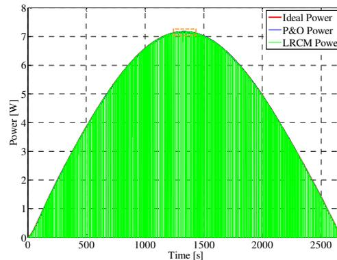
**Figure 8: Obtained PV power using P&O and LRCM**
