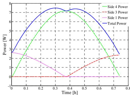
**Figure 6: Ideal power for the solar panels**
