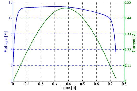
**Figure 7: Voltage and current at maximum power of side 4 solar panels**
