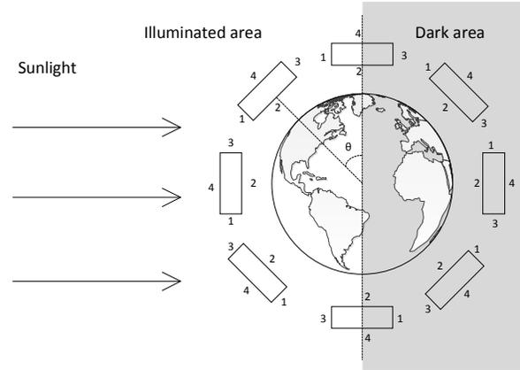
**Figure 3: Simplified orbit of a 3U Cubesat**
