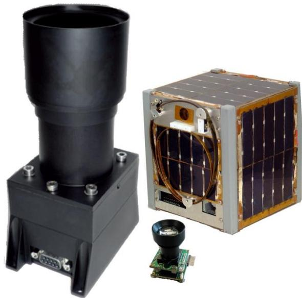
**Figure 1: ST-100 (large), ST-200 (nano) Star Trackers and CubeSat**
