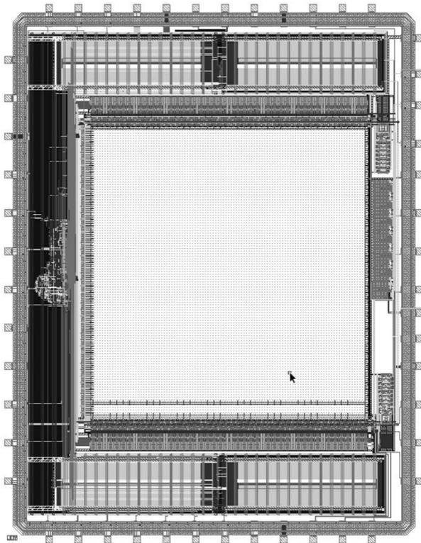
**Figure 2: CMOS photosensor 128×128 pixels**
