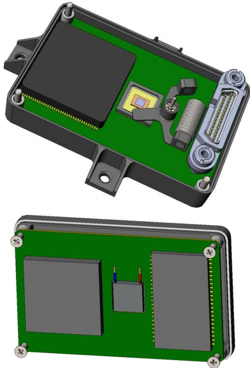
**Figure 5: Top and bottom view of the STC printed circuit board**
