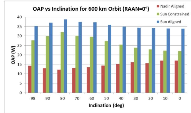
Figure 4: OAP vs Inclination for 600 km Orbit
