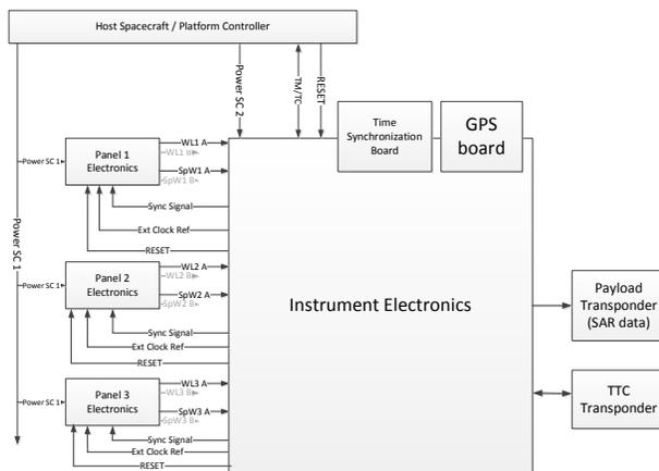
**Figure 2: Flight demonstrator architecture**
