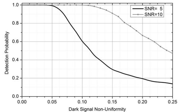
**Figure 6. Effect of dark current inhomogeneity on the star image detection**
