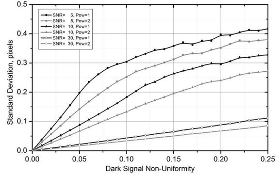
**Figure 5. Effect of dark current inhomogeneity on the position error**
