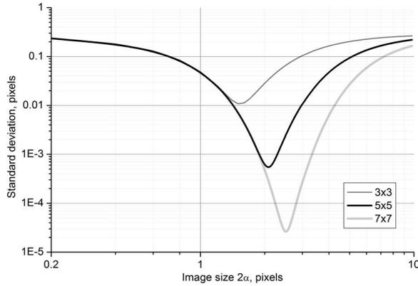
**Figure 1. Error of star image position (by formula(2)) depending on image size**
