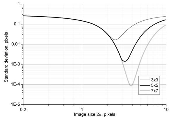
**Figure 4. Error of star image position (by formula (6)) depending on image size**
