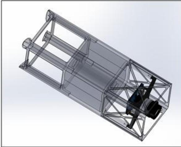
**Figure 2a: Transparent 3U CubeSat Structure**
