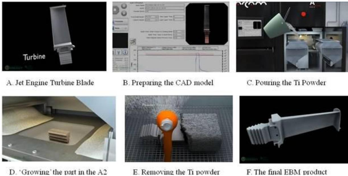
**Figure 4: ARCAM Build Sequence**
