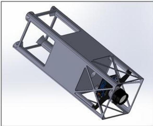
**Figure 2b: Solid 3U CubeSat Structure**
