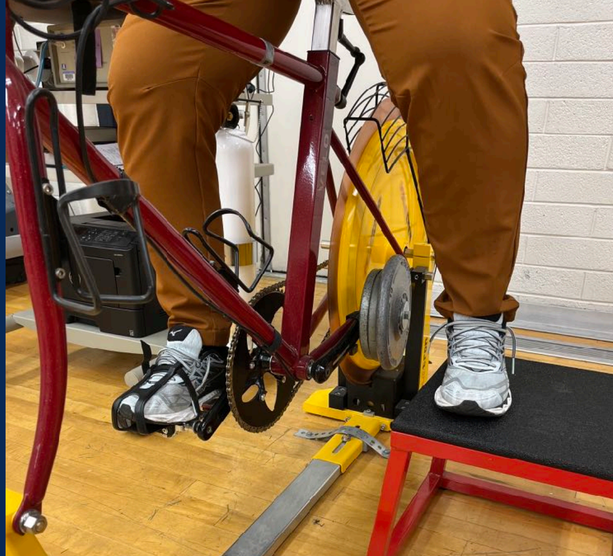
Figure 2. Right single-limb cycling design with the non-pedaling limb stabilized and counter-weight added for reduced hip flexor activation.
