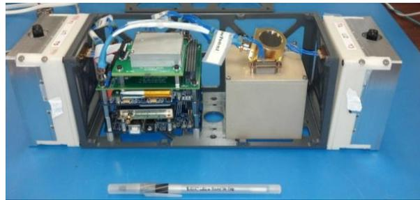
**Figure 7 - Cubesat Assembly with Hardware Before Final Integration**
