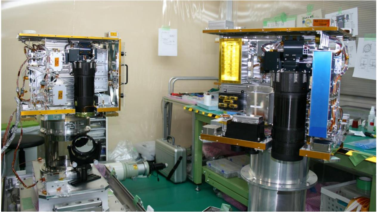
Figure 1: RISING-2 flight model (left) and RISESAT engineering model (right)
