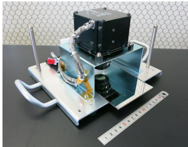
**Figure 9: Flight model of Bolometer Array.**
