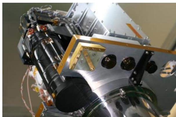
**Figure 10: Flight model of RISING-2: camera heads of HPT, LSI, and WFC from the left to right.**
