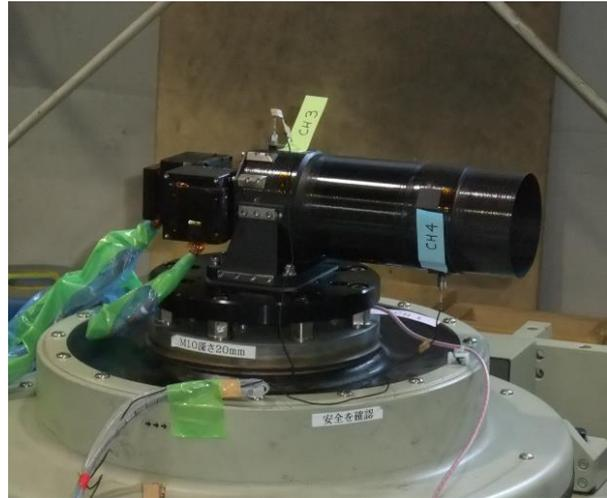
**Figure 8: Qualification vibration test of HPT.**
