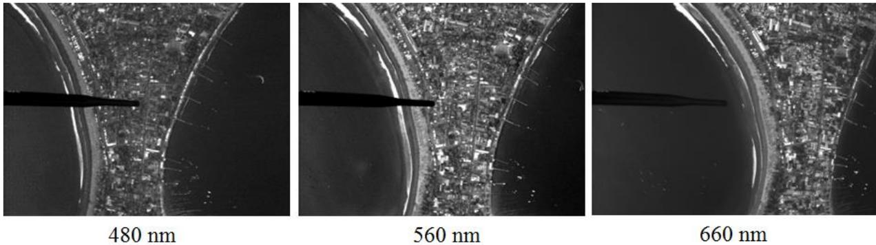
**Figure 6: Sample images taken with LCTF and the same CCD sensor in indicated three different wavelengths, taken by an UAV. A ground pixel resolution of 5m is reproduced by post image processing.**
