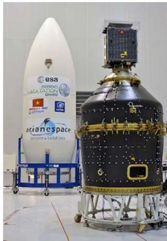
**Figure 6: Vega’s Second Launch Proba-V atop of the VESPA**
