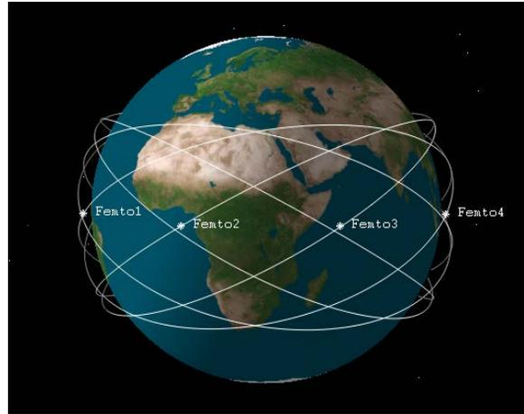
**Figure 9. Rendering of an 8 Plane 30° Inclination Constellation with One Femtosatellite Per Plane.**
