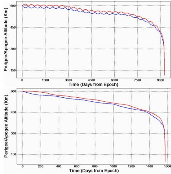
**Figure 7. Orbit Perigee and Apogee as a Function of Time for a spacecraft with a ballistic coefficient of 200  $\text{cm}^2/\text{kg}$ , (top) and 2000  $\text{cm}^2/\text{kg}$ , (bottom).**
