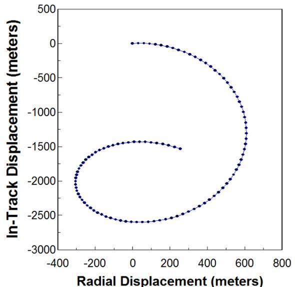
**Figure 5. Trajectory and Range Plots for a One-way Satellite Inspector Ejected at a 10° angle from the Nadir Direction at 0.5 m/s.**
