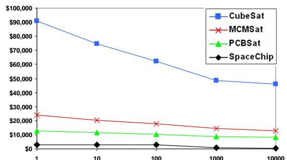
Figure 13: Unit Satellite Cost When Mass-Produced<sup>8</sup>
