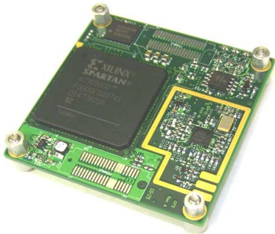
**Figure 10. Photograph of the Aerospace Corp. GPS Receiver Board. (30 grams)**
