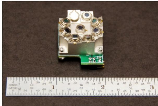
**Figure 12. Photograph of the Earth Nadir Sensor Used on the Aerospace Corporation AeroCube-4 Spacecraft.**
