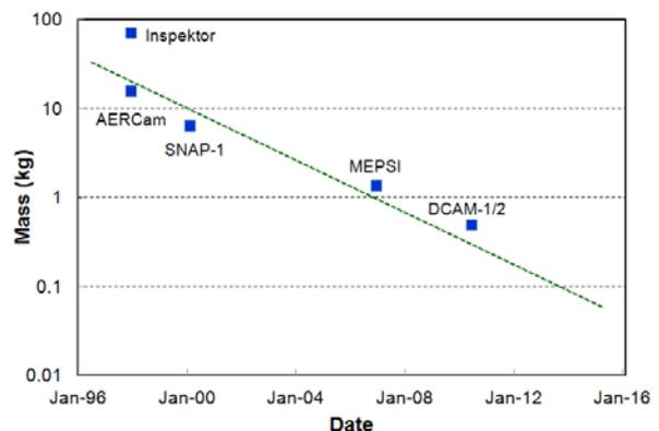
**Figure 3. Satellite Inspector Mass As a Function of Flight Date**
