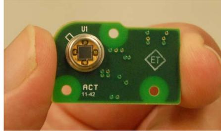
**Figure 11. Photograph of a 2-axis Sun Sensor Flown on the AeroCube-4 spacecraft. The Aperture Plate and Optical Baffle are Missing in this Photograph.**
