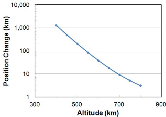
**Figure 8. Position Change, 72 hours After Changing Ballistic Coefficient from 200 cm<sup>2</sup>/kg to 2000 cm<sup>2</sup>/kg, as a Function of Circular Orbit Height.**
