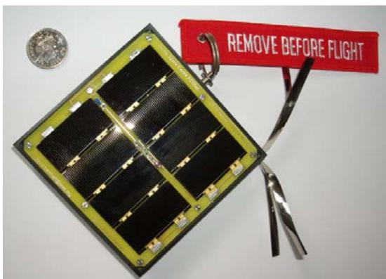
**Figure 1: Photograph of PCBSat8**
