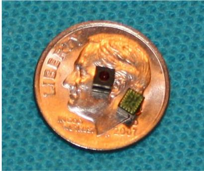
**Figure 4. Photograph of the OmniVision OVM7690 with Integrated F/3, 67° Field-of-view lens**
