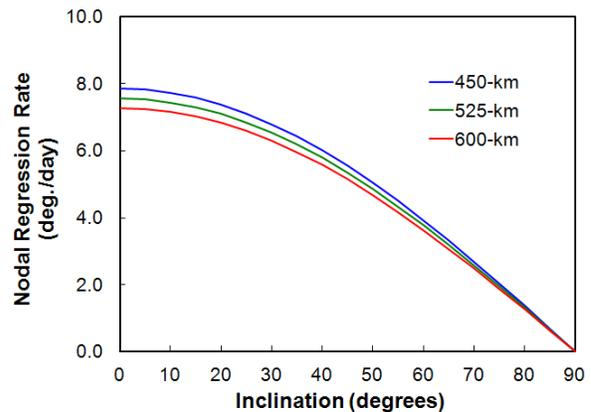
**Figure 6. Nodal Regression Rates as a Function of Orbit Inclination for Circular Orbits with 450, 525, and 600 km Altitudes.**
