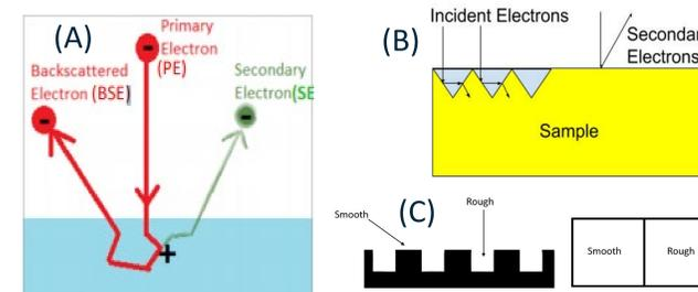
Fig 4. (A) Diagram showing incident primary electrons, emitted backscattered electrons and secondary electrons (B) how roughness influences electron emission (C) the sum of rough and smooth sections are used in the patch model for Electron Yield.
