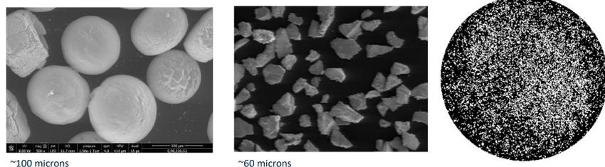
Fig 2. An example of a SEM image, (left and center) and the composite formed from the sum of several overlapping SEM images (right).
