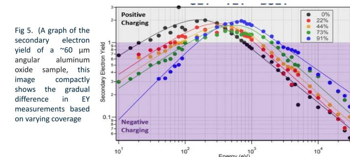
Fig 5. (A graph of the secondary electron yield of a  $\sim 60\ \mu\text{m}$  angular aluminum oxide sample, this image compactly shows the gradual difference in EY measurements based on varying coverage
