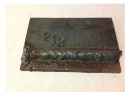
Figure 6. SMAW weld test coupon.
