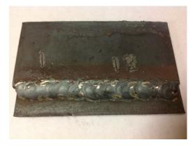
Figure 2. Weld test coupon.
