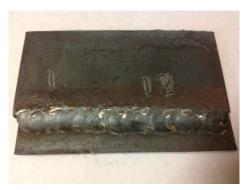
Figure 5. GMAW weld test coupon.
