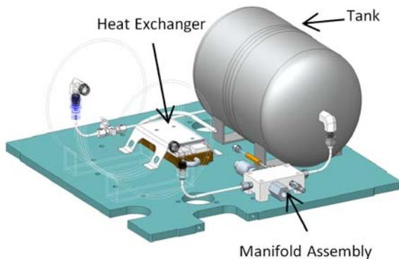
**Figure 3: CAD model of propulsion system assembly**
