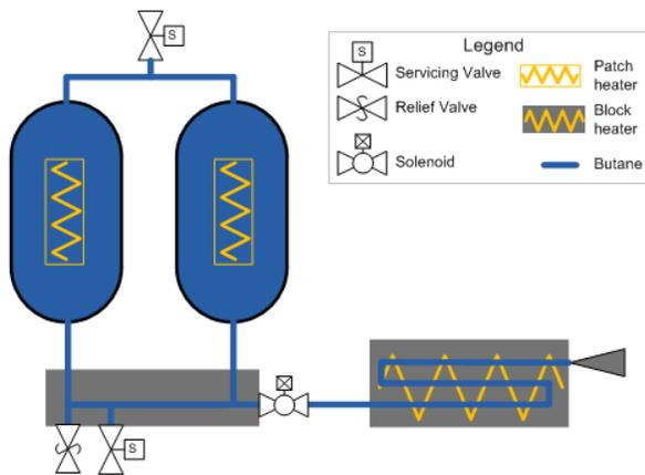
**Figure 2: Propulsion system schematic diagram**
