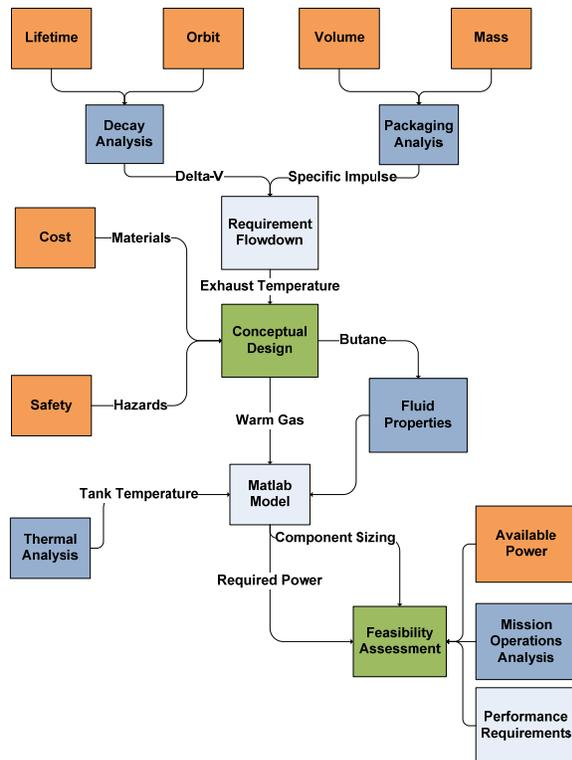
Figure 1: Overall design flow
