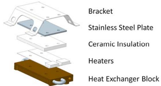
**Figure 6: Exploded view of heat exchanger assembly**
