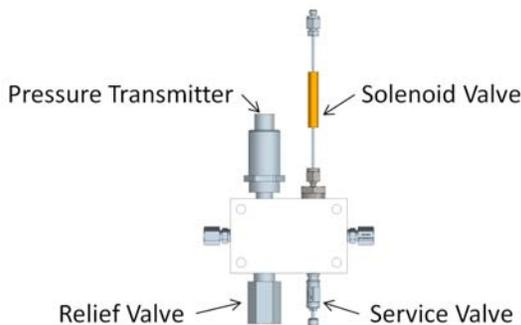
**Figure 5: Diagram of manifold assembly**
