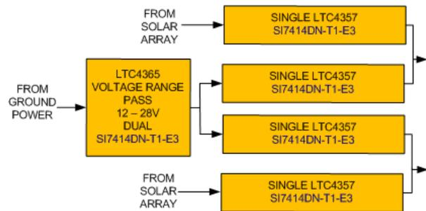
Figure 3: Ground Power Detail
