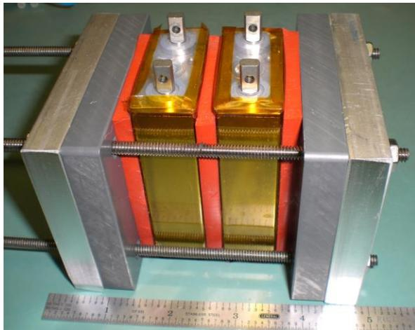
**Figure 6: Battery Cells in Shipping Fixture**
