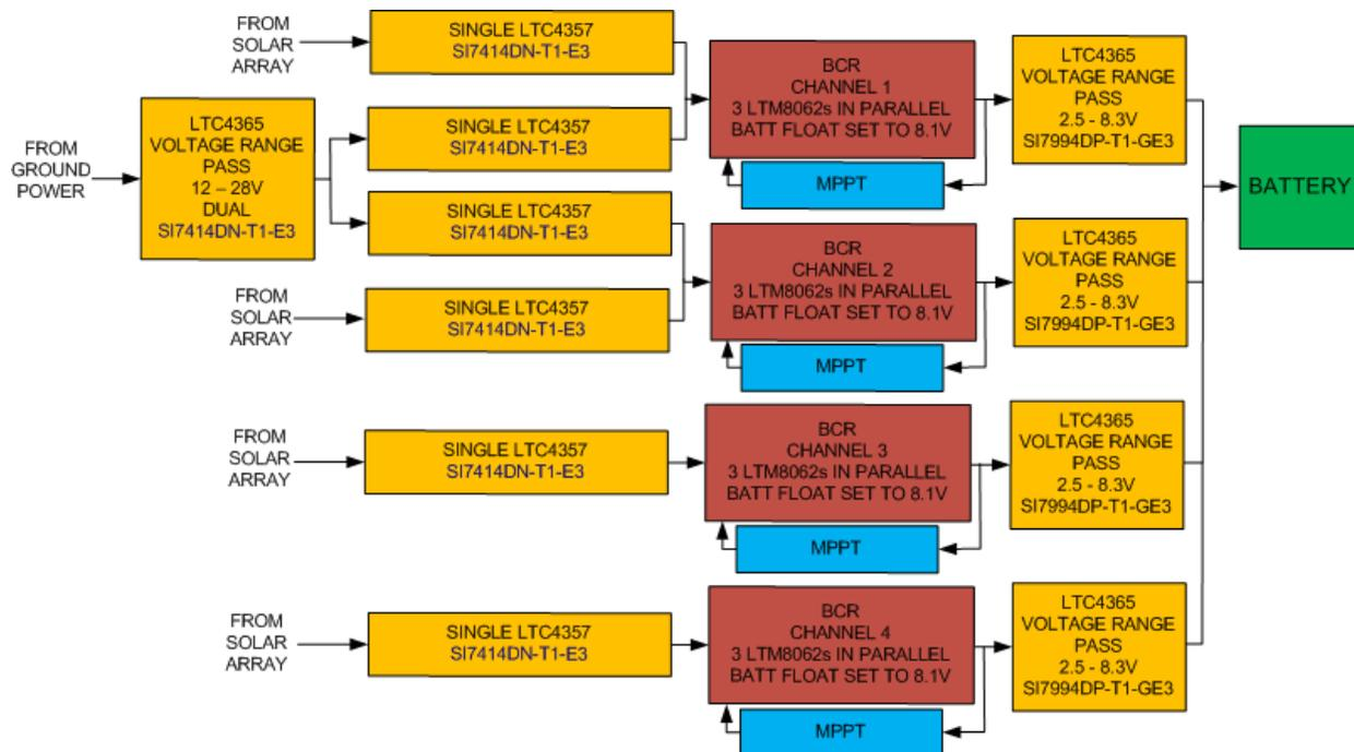
**Figure 2: Solar Panel to Battery Power Flow**
