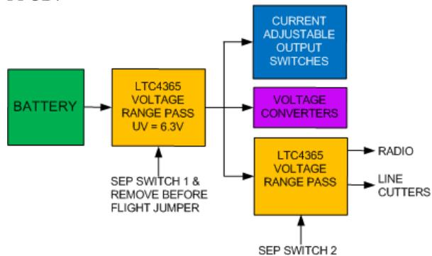
**Figure 4: Separation Switches and Remove Before Flight Jumper**
