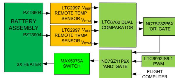
**Figure 8: Battery Heater Circuit**
