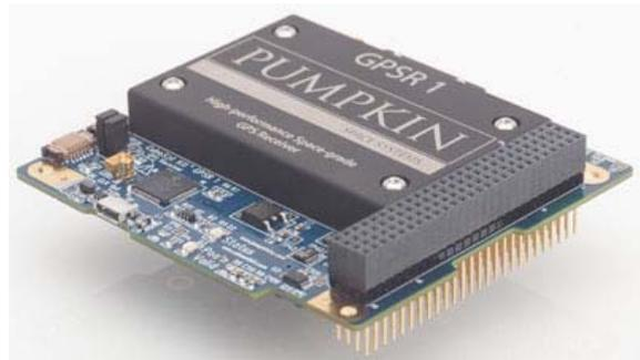
Figure 1: GPSRM 1 Module
