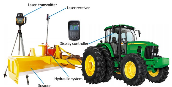
Figure 3. Example of laser land leveling system ( http://www.shtbag.com/productsInfoEng.html ).
