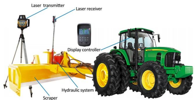
**Figure 3.** Example of laser land leveling system (<http://www.shtbag.com/productsInfoEng.html>).
