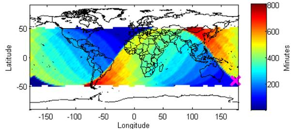
**Figure 6. Average Time Since Last Pass (TSLP) for a satellite in 51.6° inclination, 500 km orbit and a single ground station located in New Zealand (ground station location indicated with the X).**
