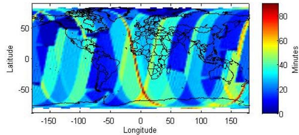
**Figure 11. Average TTNP between a satellite in 500 km circular sun synchronous orbit and the ground stations shown in Figure 8.**
