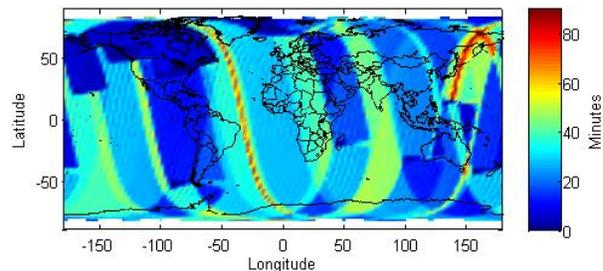
**Figure 12. Average TSLP between a satellite in 500 km circular sun synchronous orbit and the ground stations shown in Figure 8.**
