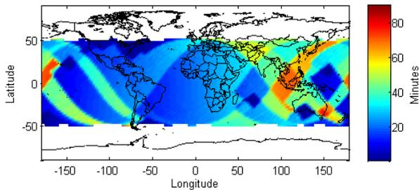
**Figure 10. Average TSLP between a satellite in 51.6° inclination 500 km circular orbit and the ground stations shown in Figure 8.**
