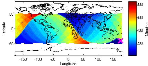
**Figure 5. Average Time To Next Pass (TTNP) for a satellite in 51.6° inclination 500 km circular orbit and a single ground station located in New Zealand (ground station location indicated with the X).**
