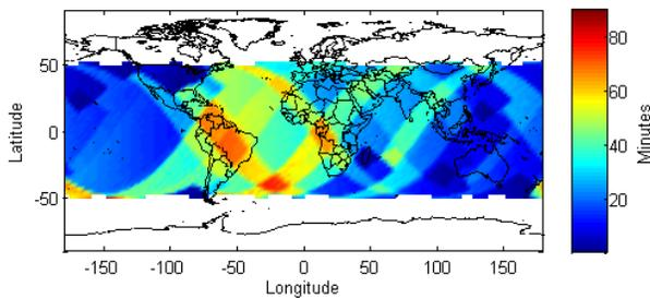
**Figure 9. Average TTNP between a satellite in 51.6° inclination 500 km circular orbit and the ground stations shown in Figure 8.**
