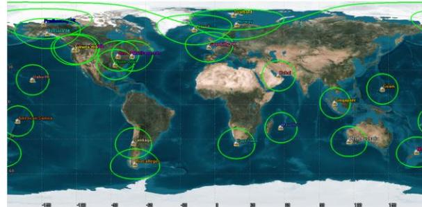
**Figure 7. Initial candidate ground station locations used to evaluate different configurations of ground station grouping. The visibility is shown to spacecraft in 450 km altitude orbit.**
