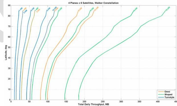
**Figure 3. Small constellation ( $\leq 25$  satellites) average daily throughput for a 4x6 constellation geometry and the analyzed different spacecraft transmit antenna/power configurations.**
