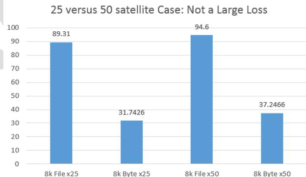
**Figure 4 – A constellation size of 25 satellites does not impact performance at this data volume size.**
