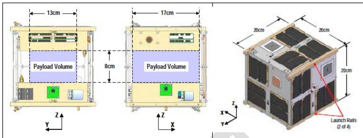
**Figure 6. Larger form-factor nanosatellites offer additional hosted payload capacity above what is needed for the Outernet broadcast service [images credit: UTIAS/SFL].**
