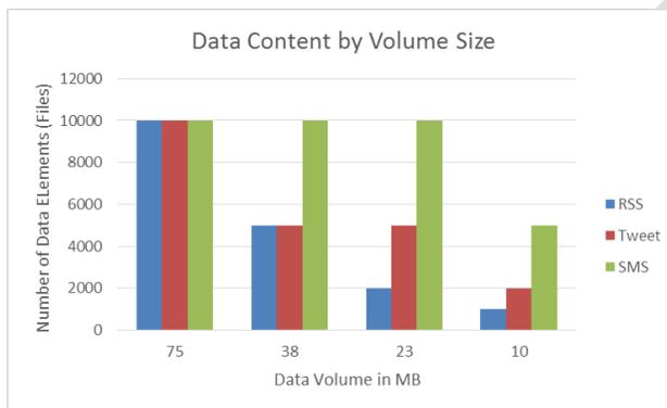
**Figure 5 - Lower data rates require a change in the overall user content.**
