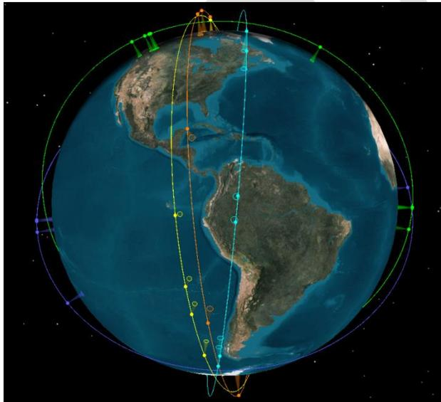
**Figure 2. Random (Monte-Carlo) constellation layout. The planes are randomly distributed about the north pole, and the satellites are randomly spaced within each plane.**
