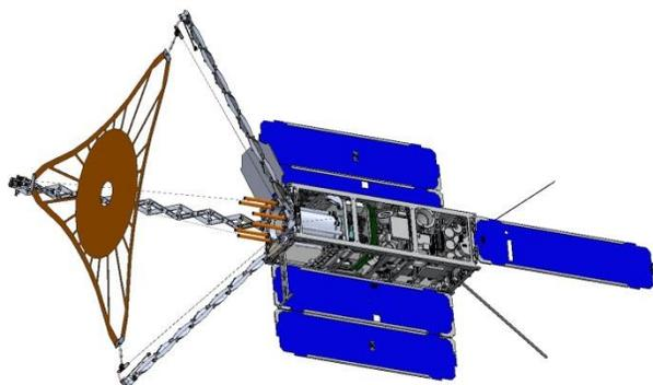
**Figure 1: FalconSAT-7 Deployed Configuration**
