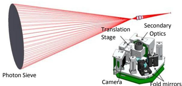
**Figure 2: Zemax model of the optical system (left) and CAD model (right) of the optical platform**
