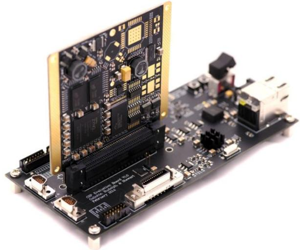
**Figure 2: CSPv1 Mated with Evaluation Board**
