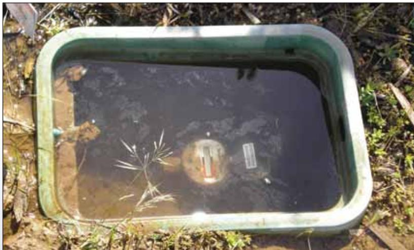
This experimental fluidic-oscillation-type meter in Utah's Weber Basin Conservancy District had a cracked and leaking base plate, which was likely the result of freezing. Despite the leak and submersion the meter was still registering flow.
