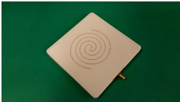
**Figure 11. An embedded two-arm Archimedean spiral.**
