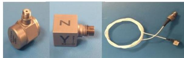
Figure 4. Dytran accelerometers used in the demonstration.
