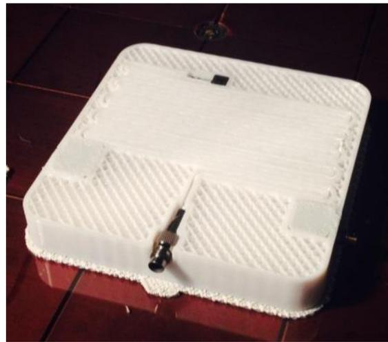
**(b) 3D-printed caps installed above larger sensors.**
