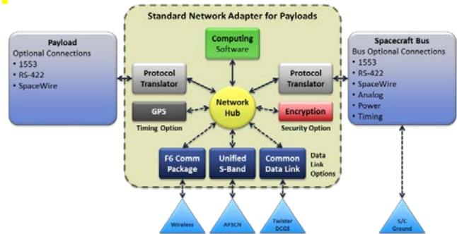
Figure 3 The SNAP Demonstration Overview<sup>9</sup>
