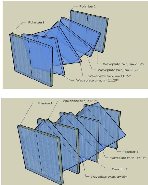
**Figure 11.** The Lyot spectral filter (top) and Solc spectral filter (bottom).
