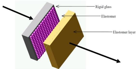
**Figure 13.** Schematic of a Elastomer Fabry Perot Etalon Array.
