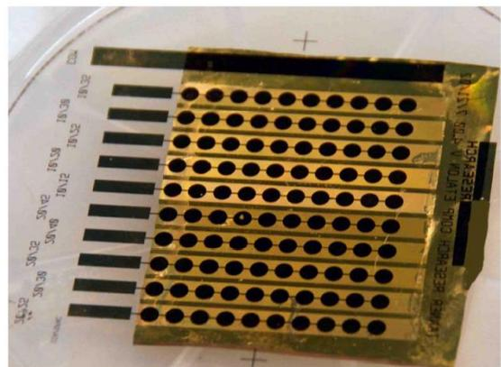
**Figure 14** 16 x 16 Array of Elastomer Fabry Perot Etalons.
