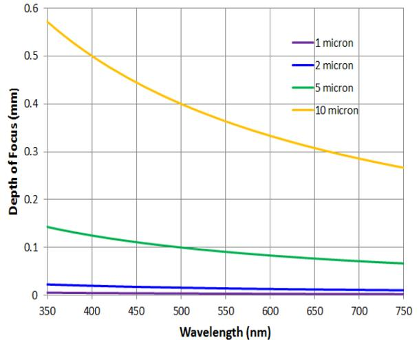
**Figure 4.** Depth of Focus of Optical Sieve.
