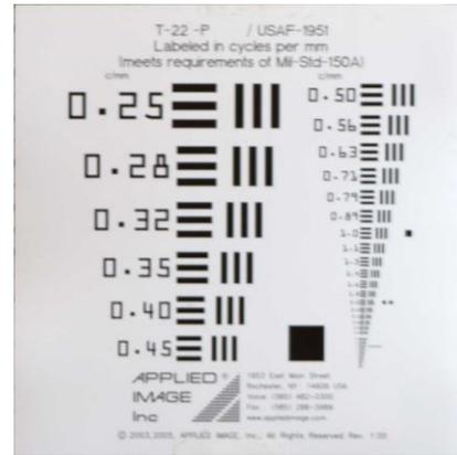
**Figure 7.** Image of a USAF tri-bar test pattern produced by our diffractive telescope system.
