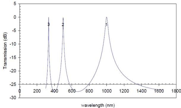
**Figure 15.** Spectral Transmission of Fabry Perot Etalons.
