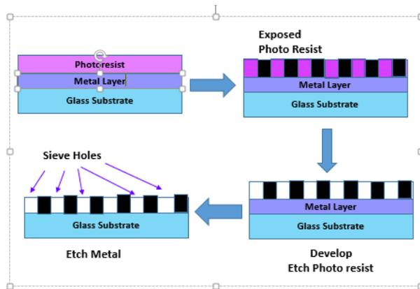
**Figure 5.** Schematic of the optical sieve fabrication process.
