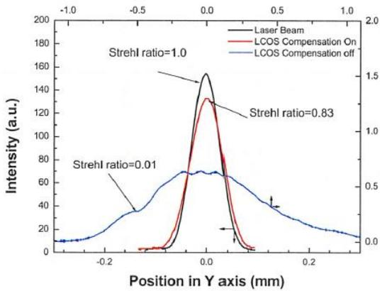
**Figure 10.** Beam profile of a focused laser beam.
