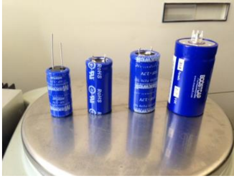
Figure 6: Tested super-capacitors from Maxwell Technologies, Inc. Sizes range from 50F (Left) to 310F (Right).
