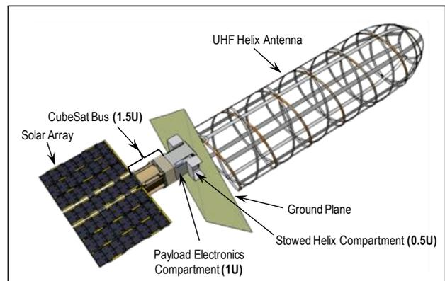
**Figure 15: Conceptual Cubesat Using the Deployable UHF Antenna System**
