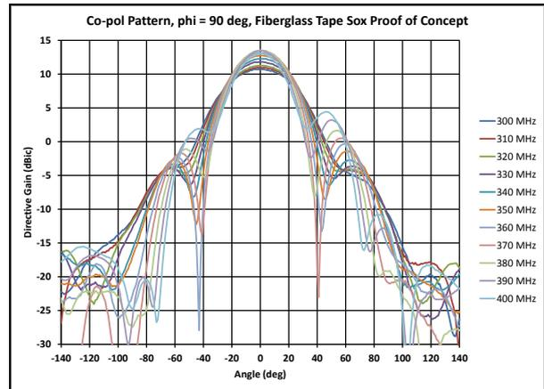
**Figure 11: Co-polar Radiation pattern of the Deployable Helix at Multiple Frequencies**
