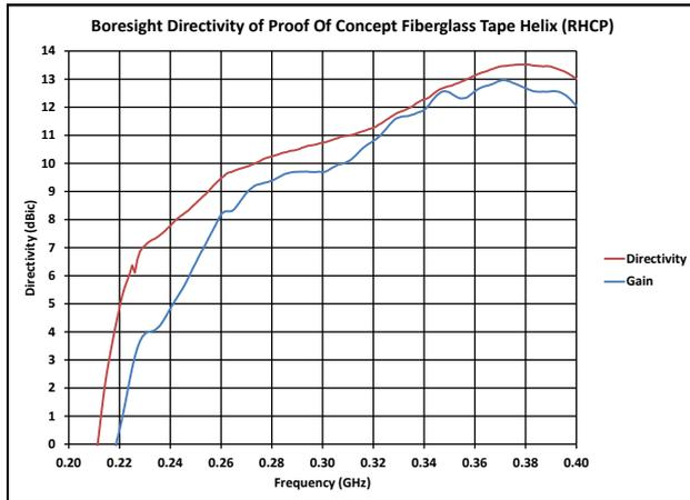
**Figure 13: Deployable Helix Gain and Directivity Relative to an Ideal Circular Polarized Incident**
