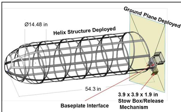
**Figure 5: Deployed Antenna System**
