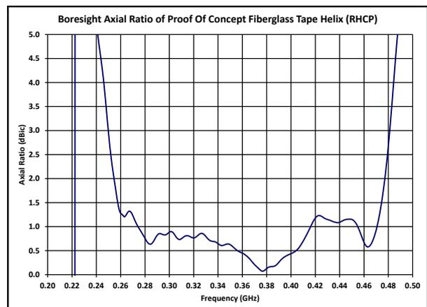
**Figure 12: Axial Ratio of the Deployable Helix**
