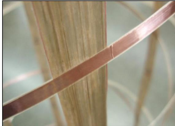
**Figure 2: Copper Conductor Element Attached to A Single Helical Element**
