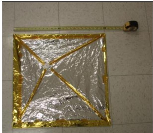
**Figure 3: Deployed Ground Plane**
