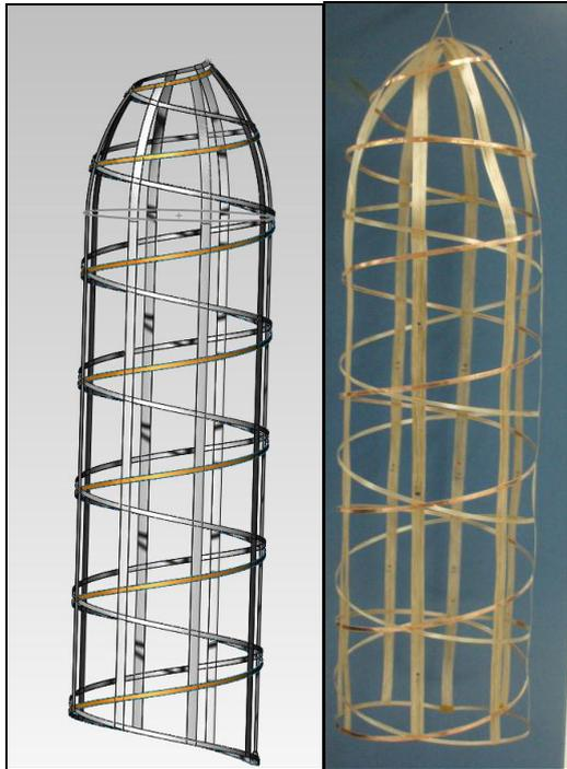
**Figure 1: Deployed Helix as Designed and Constructed**
