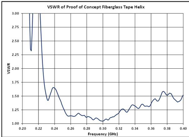
**Figure 9: VSWR of the Deployable Helix**
