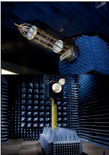
**Figure 10: Deployable Helix Under Test**
