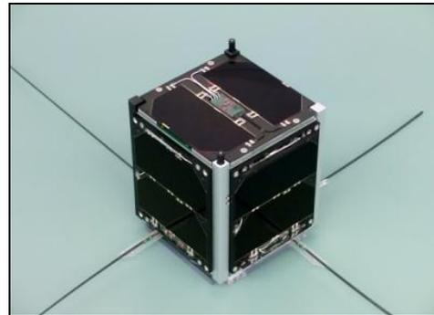
**Figure 14: Standard 0dBi Tape Spring Antenna**
