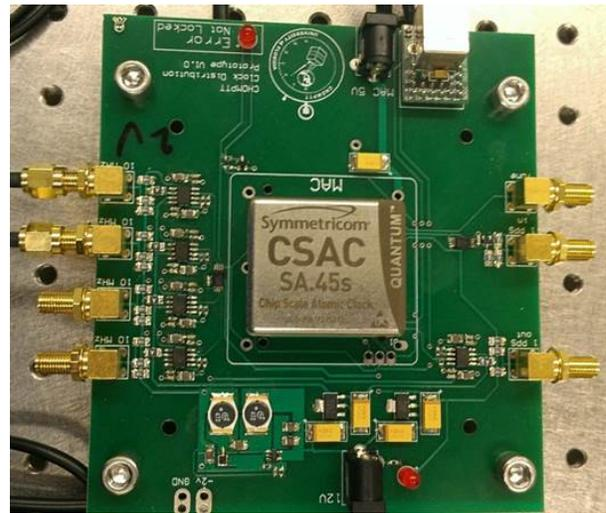
**Figure 2: Chip Scale Atomic Clock and breadboard version of the OPTI clock distribution electronics**
