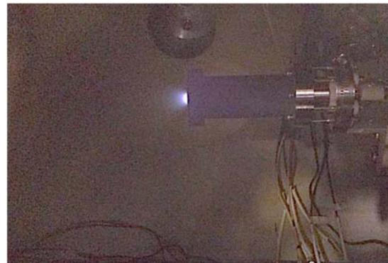
Figure 2: The LaB<sub>6</sub> hollow cathode and the plasma plume
