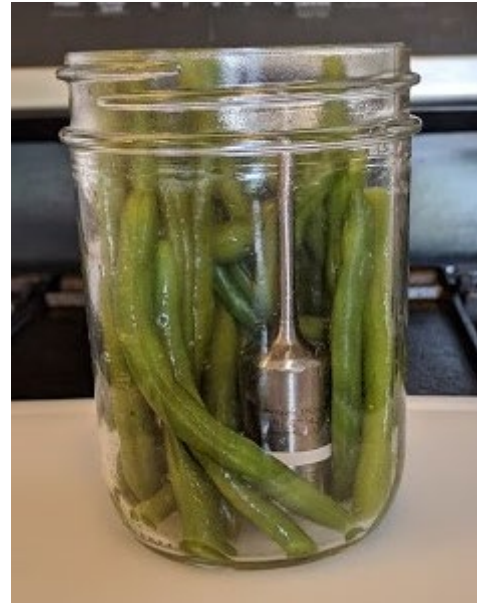
Picture of data logger in jar of green beans
