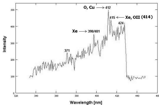
**Figure 10.—Glow spectrum in a xenon plasma.
