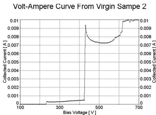
Figure 7.—Gaseous discharge begins at about 430V potential.
