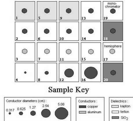
Figure 1.—Sample coupon testbed used in snapover experiments.
