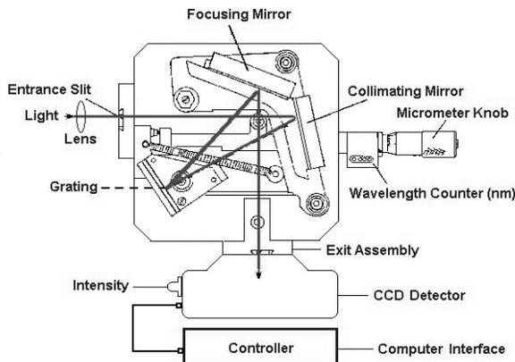
Figure 2(a).—Spectrometer setup used in analyzing snapover-induced glow.
