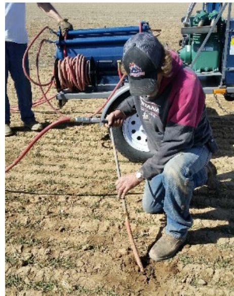
Using PERC machine to fumigate squirrels.
