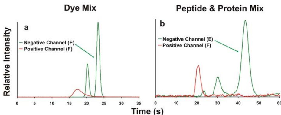
**Fig. 4** Representative electropherograms of the separations performed on the PEG coated (low EOF) microfluidic device. Sample injection from a central channel is achieved, and anions and cations are separated in different channels. An electropherogram of the fluorescent dye mixture is shown in (a), and an electropherogram of the protein and peptide mixture is shown in (b). Each component was baseline resolved with high efficiencies in <1 minute.
