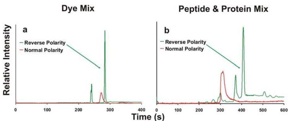
**Fig. 6** Representative electropherograms of the separations performed with CE on a PEG coated fused silica capillary with reduced EOF. Two injections using opposite polarities between the separations are required because of the reduced EOF. In (a), the separation of the fluorescent dye mixture is shown, and in (b), the separation of a protein and peptide mixture is shown.
