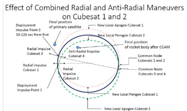
**Figure 2: Separation scheme optimization to avoid spacecraft re-contact**
