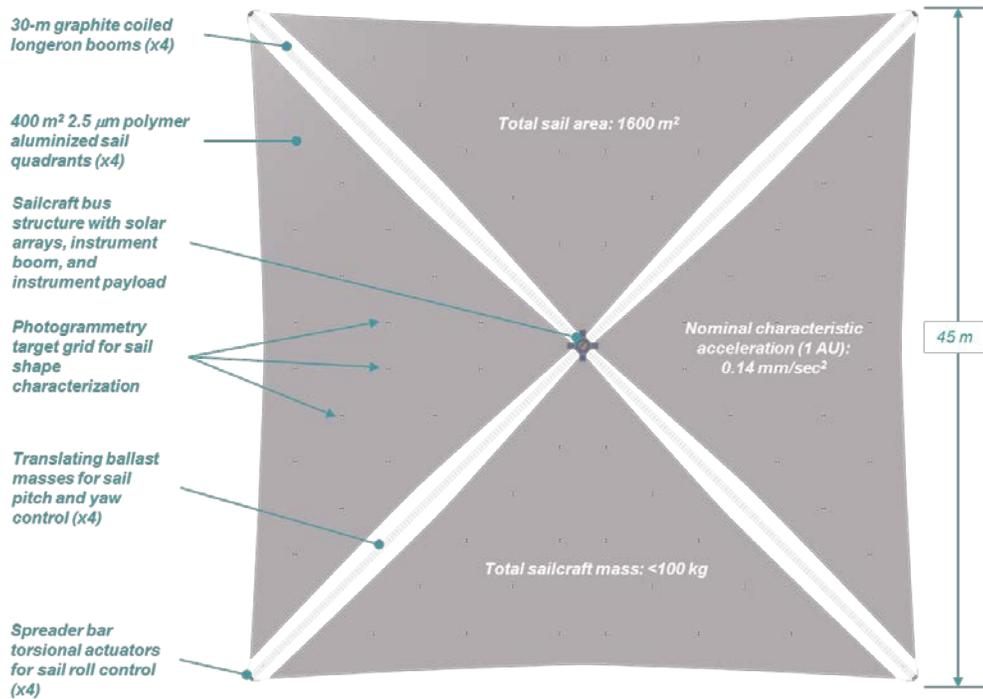
Figure 8: Deployed solar sail characteristics. Total sail area is 1600 m<sup>2</sup>. Total sailcraft mass is < 100 kg.
