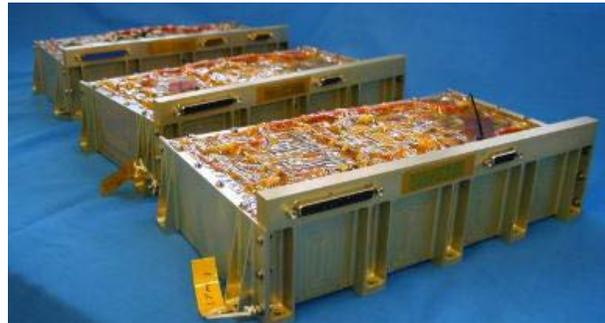
**Figure 18: 24Ah modular battery building block**
