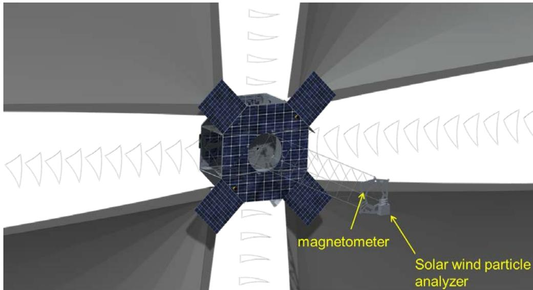
**Figure 9: Solar Sail Technology Demonstration Mission particles and fields instruments**
