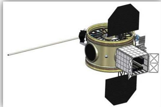
**Figure 5: OMV with Space Weather Payloads and FANTM-RiDE Smallsat Dispenser**
