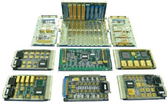
**Figure 15: Moog Integrated Avionics Unit**
