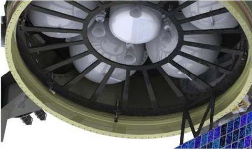
**Figure 19: OMV Propulsion Tanks and Thrusters**
