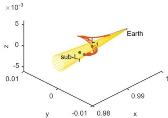
**Figure 10: Solar Sail Technology Demonstration Mission sub-L1 Artificial Lagrange Point destination, with 5 degree sun exclusion cone indicated.**
