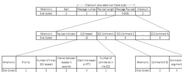
**Figure 9: Stored Command Sequence Message Structure**
