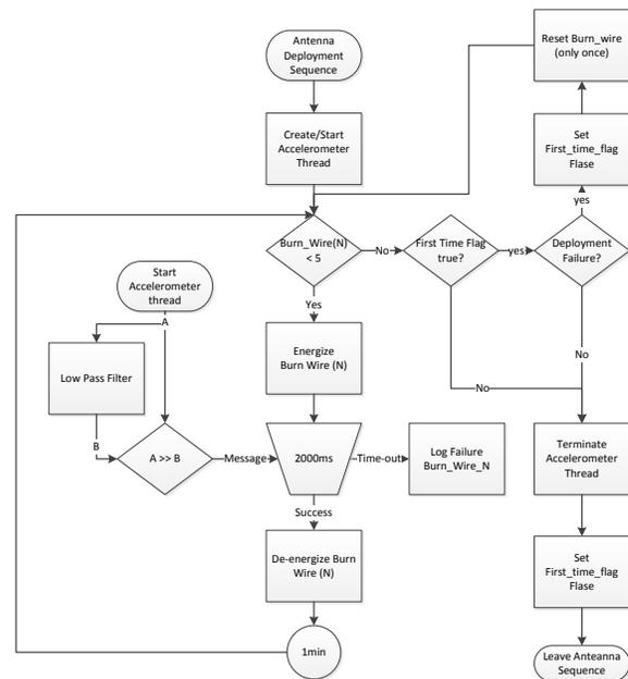
**Figure 6: Antenna Deployment Sequence Diagram**
