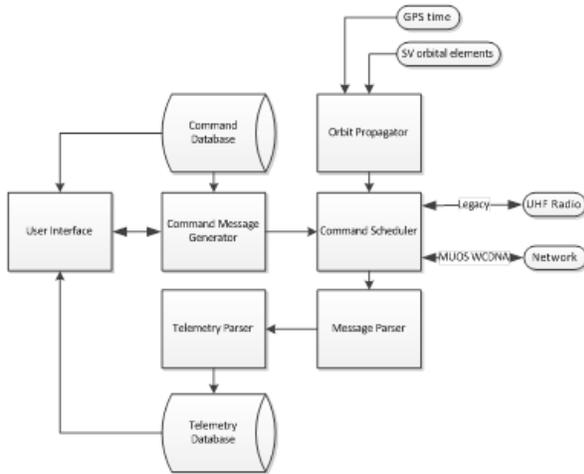
**Figure 7: Ground Software Architecture**
