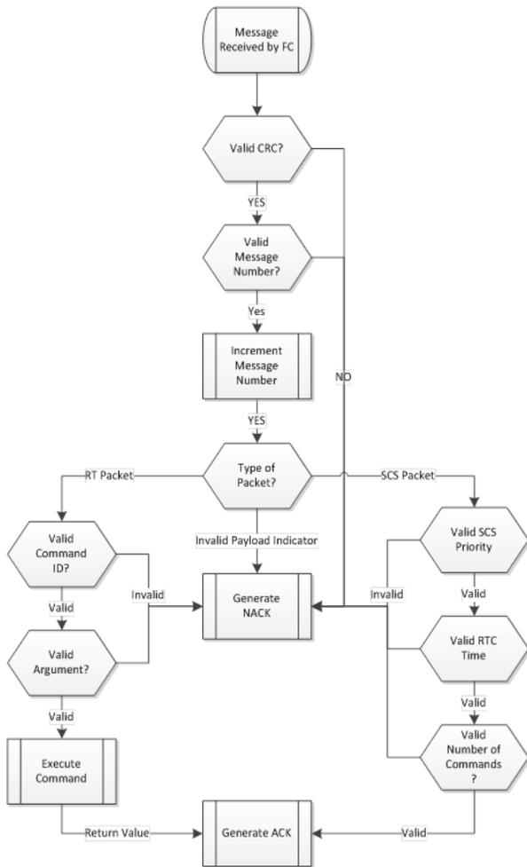
**Figure 8: ACK/NACK Generation Logic**
