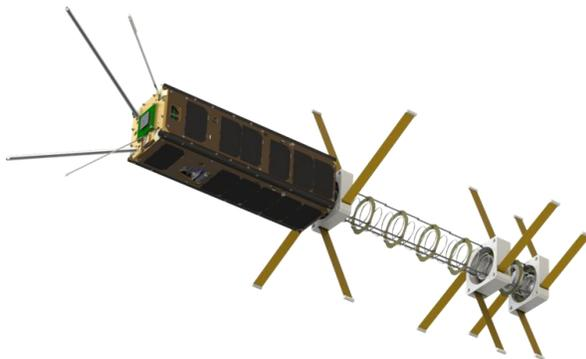
**Figure 3: ICE-Cap CubeSat Image with Both Antennas Deployed**
