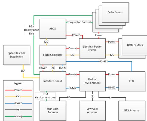
**Figure 4: ICE-Cap Interface Architecture**
